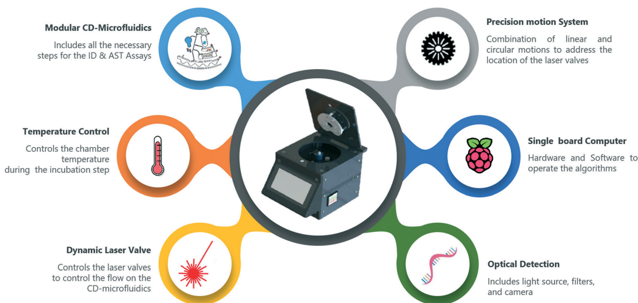
Fig. 1 The SpinBox design and components.
